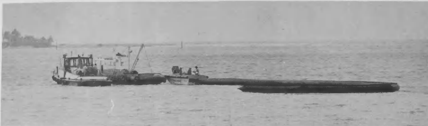
The Seapack, a 23-ft fiberglass boat releases a boom which is automatically inflated. The boom surrounds a "spill" for recovery by the Seaskimmer shown below.
